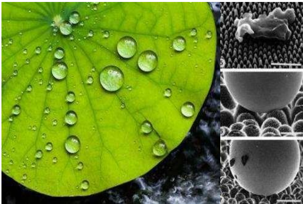
lotus leaf superhydrophobic structure
